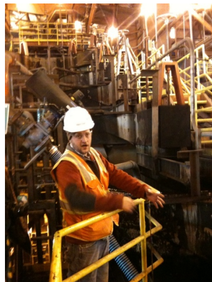
In this photo, we are inside the gold recovery plant. Matt is standing next to a series of large tanks filled with a mixture of the gold-cyanide solution and powdered activated carbon (PAC). The PAC is made from burnt coconut husks and after the solution is circulated long enough to extract the gold, it is filtered and a gold-rich carbon mud is the end result of the leaching process. Unfortunately pours of molten gold that occur after the mud is combusted are done during the weekdays, so we missed out on seeing the final product!
