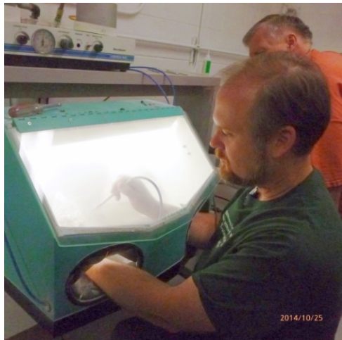
Rob Lorda demos an air abrasive cleaning tool
