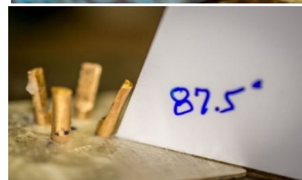
Figure 9: Prongs just after soldering into position, coloring is from melted flux and is chemically removed.
