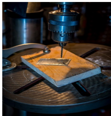
Figure 8: Drilling the holes with a drill press at 87.5° for the prongs.
