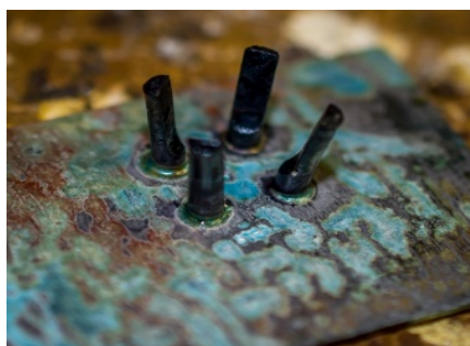
Figure 7: Roughed out gold-filled wire prongs for the Libyan Desert glass, and the prefabricated prong finding that was used as a model.
