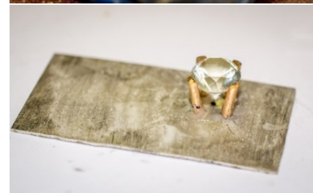
Figure 10: Prongs polished, and knotted to capture the girdle of the stone. Stone temporarily set on the prongs.
