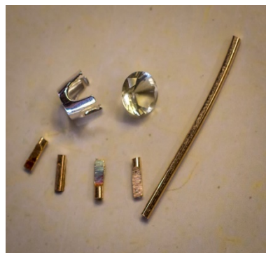
Figure 7: Roughed out gold-filled wire prongs for the Libyan Desert glass, and the prefabricated prong finding that was used as a model.
