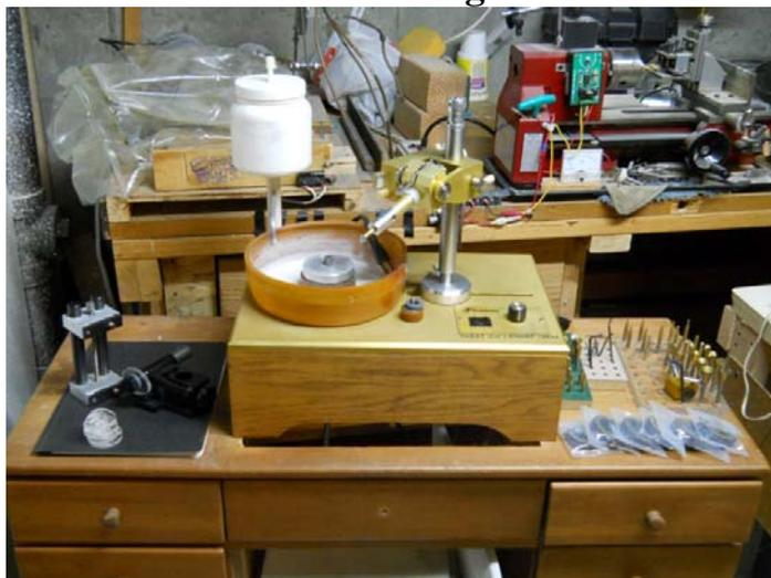
Facetron faceting machine, complete, with needle stop. Accessories include:
